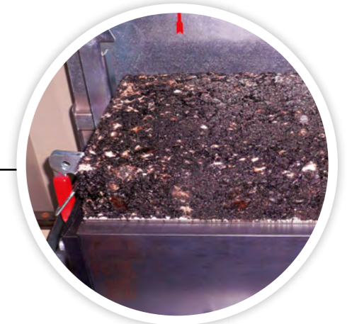
Asphalt sample moved upward for demoulding
